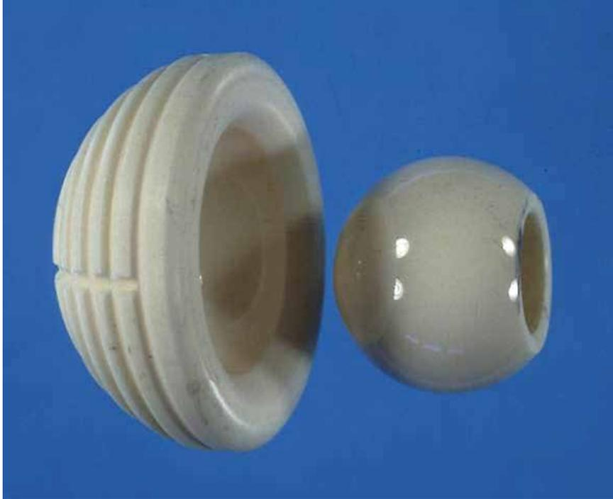
Figure 4 - Couple alumine-alumine
