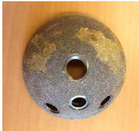
Figure 16 - Cotyle type press-fit
